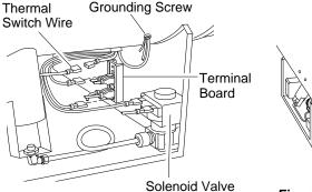
Figure 6 - Location of Motor Wires
